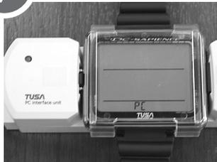
Ensure that the single connection pin on the underside of this unit contacts securely with the connection port of the IQ-800 and that PC mode is displayed on the screen of the IQ-800.
