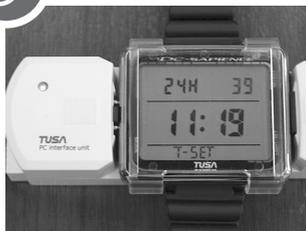
Once the log data has been transferred, the IQ-800 will switch into T-SET mode and the red light will come on.
