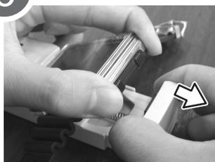
Press down on the IQ-800 and extend the holder part of the PC Interface Unit, then set the IQ-800 into place as shown in the photograph to the left.
