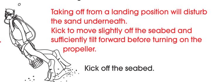
⑥ After moving away from the seabed with the entire body tilted forward to around a 45-degree angle, pull the throttle lever for takeoff.
